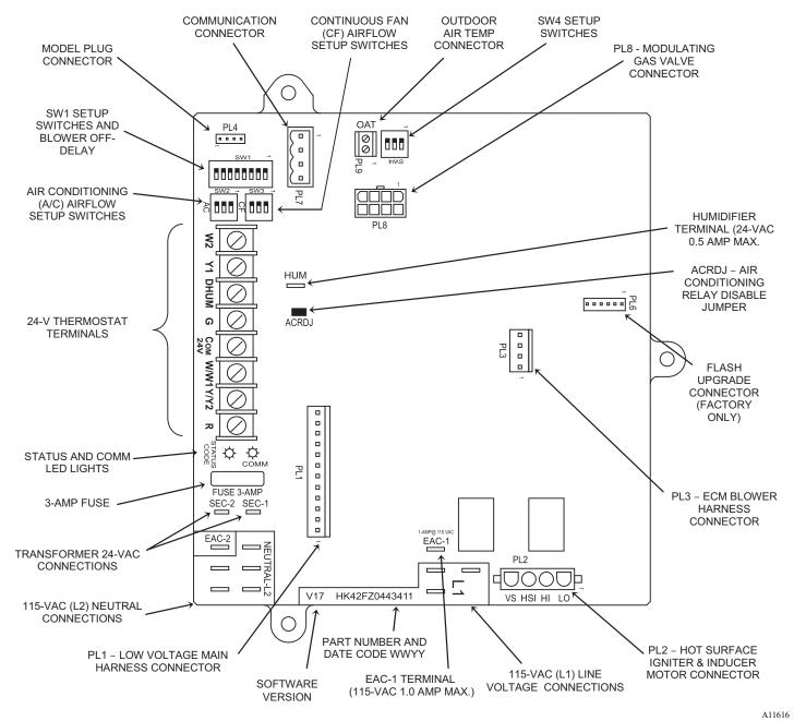
Fig. 37 - Example of Modulating Furnace Control
