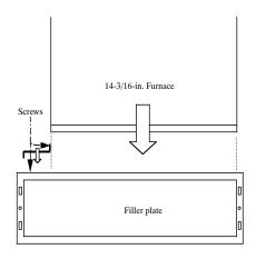
14-3/16-in. Furnace with Filler Plates, Off-Set to Right
