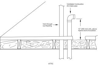
${\bf Fig.~47-Vent~Terminations~for~Ventilated~Combustion~Air} \\ {\bf Size~the~Vent~and~Combustion~Air~Pipes}$
