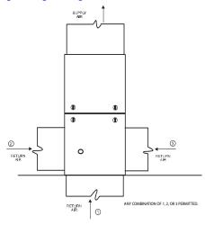
Fig. 20 – Upflow Return Air Configurations and Restrictions  $^{\rm A11036}$
