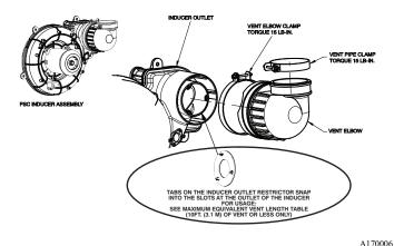
Fig. 53 – Inducer Vent Elbow (Appearance May Vary)
