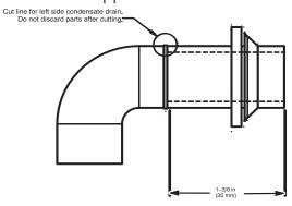
Fig. 16 – Modify Rubber Drain Elbow
