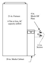
Media Cabinet Installation Option for 4-Ton or Less A/C Capacity
