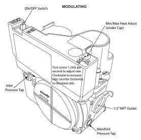
Fig. 64 - Gas Valve without Tower Pressure Ports
