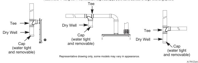
Fig. 51 – Recommended Combustion Air Inlet Moisture Trap
