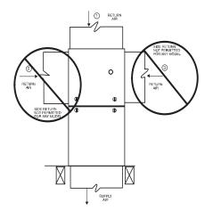
Fig. 21 - Downflow Return Air Configurations and Restrictions
