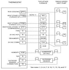
Modulating and 2-Stage Furnace with Single-Speed Heat Pump
