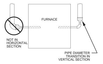
Fig. 48 – Combustion Air and Vent Pipe Diameter Transition A93034 Location and Elbow Configuration
