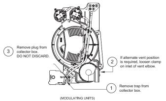
Unconverted Factory Trap Configuration
