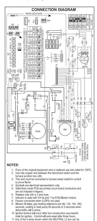
connected to any terminal within the box.
