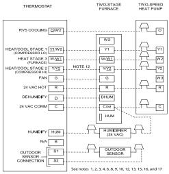
Modulating and 2-Stage Furnace with Two-Speed Heat Pump
