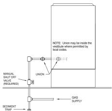
Fig. 31 – Typical Gas Pipe Arrangement
