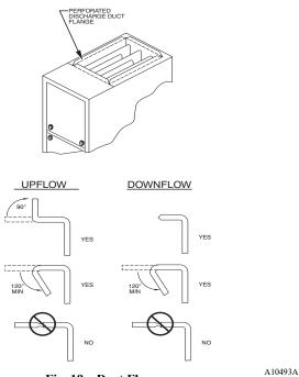
Fig. 19 - Duct Flanges
