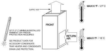
Fig. 3 – Freeze Protection and Return Air Temperature
