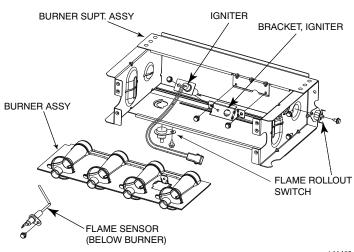
Fig. 69 – Burner Assembly
