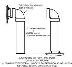
Fig. 45 – Combustion Air Pipe Attachment
