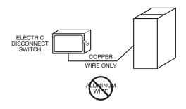
Fig. 33 – Field-Supplied External Electrical Box on Furnace Casing **J-Box Installation**
