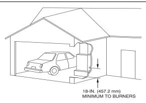
Fig. 5 – Installation in a Garage
