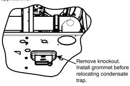
Fig. 17 – Horizontal Drain Trap Grommet
