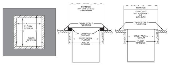
Fig. 24 – Installation on Combustible Flooring
