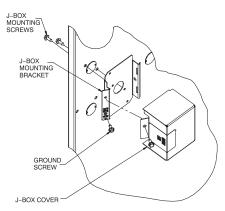
Fig. 34 – Installing J-Box (When Used) Appearance May Vary
