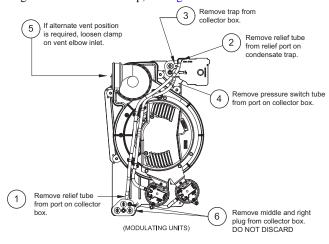
Unconverted Factory Trap Configuration
