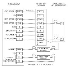
Modulating and 2-Stage Furnace with Single-Speed Air Conditioner
