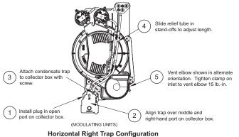
Fig. 10 – Horizontal Right Trap Configuration (Appearance May Vary)
