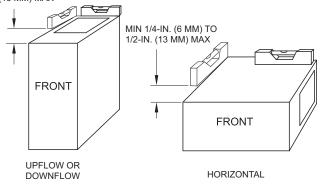
Fig. 18 – Furnace Pitch Requirements
