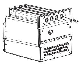
Fig. 72 – Cleaning Heat Exchanger Cell
