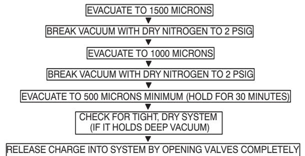
**Fig. 26 — Triple Evacuation Method**
