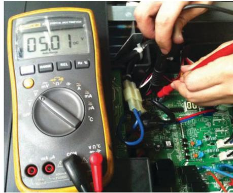
**Fig. 49 — Test the voltage**
