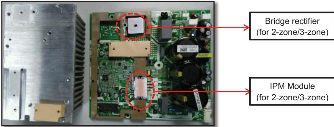
**Fig. 54 — Bridge Rectifier (for 2-zone/3-zone) and IPM Module (for 2-zone/3-zone)**
