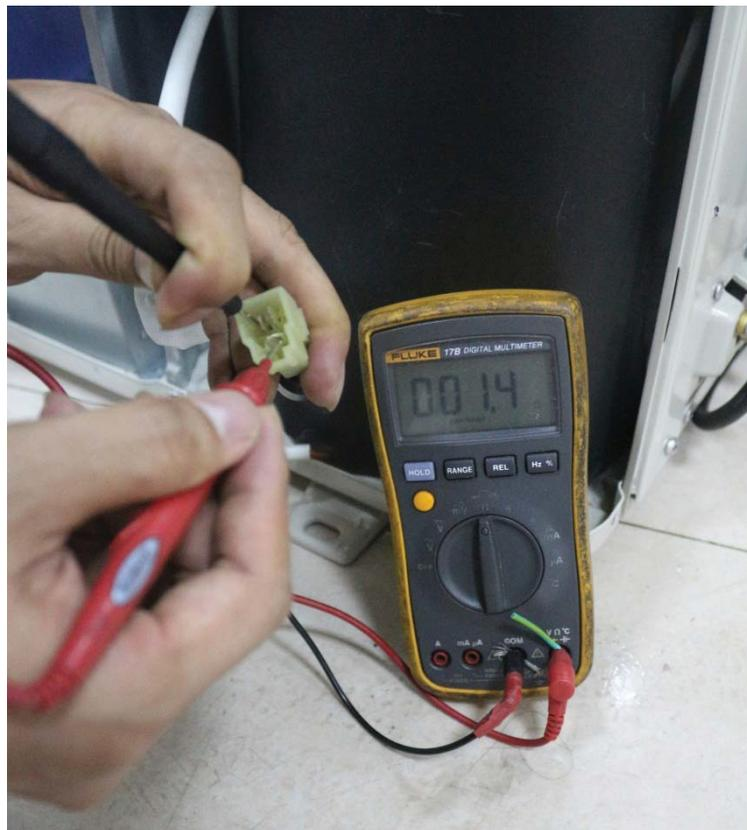
**Fig. 69 — Test the voltage**
