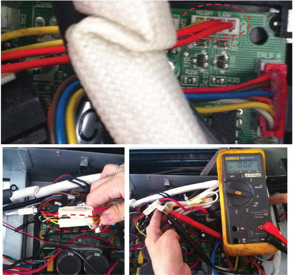
Fig. 64 —Test the voltage
