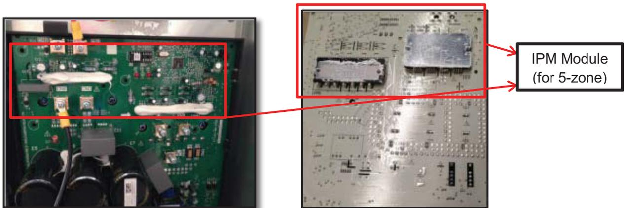
Fig. 57 — IPM Module (for 5 - zone)
