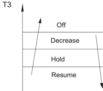
**Fig. 30 — High Condenser Coil Temperature Protection**
