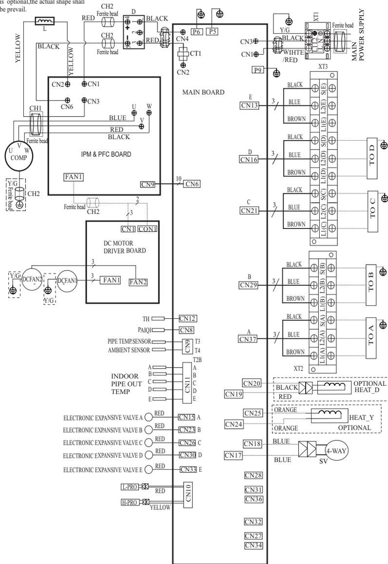
**Fig. 17 — Wiring Diagram 36K - 4 Zone Max**
