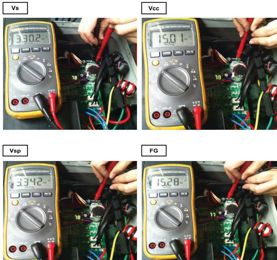
Fig. 61 —Test the Voltage
