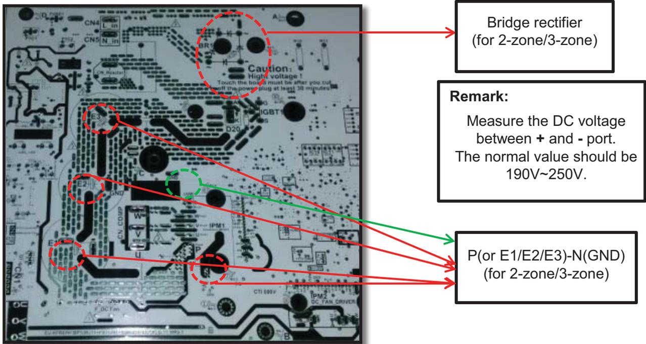
Fig. 53 — Bridge rectifier (for 2-zone/3-zone)
