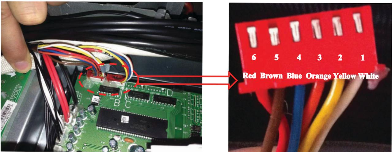
Fig. 74 — Disconnect the connectors
