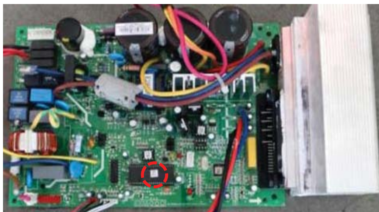
Fig. 22 – Outdoor PCB (18K Model)
