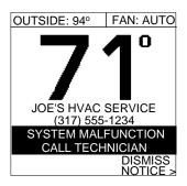
This message may be generated from any of the communicating system components, and will be displayed as shown in Figure 2. The following events may generate this message:
