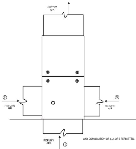
Fig. 20 – Upflow Return Air Configurations and Restrictions
