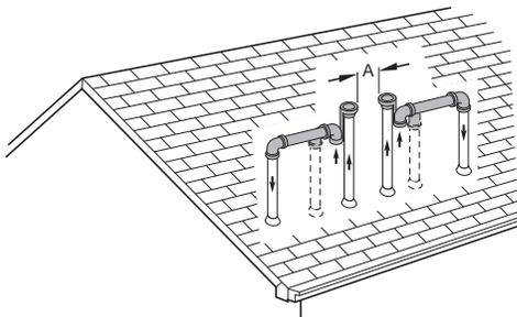
**Fig. 46 – Pipe Vent and Combustion**
