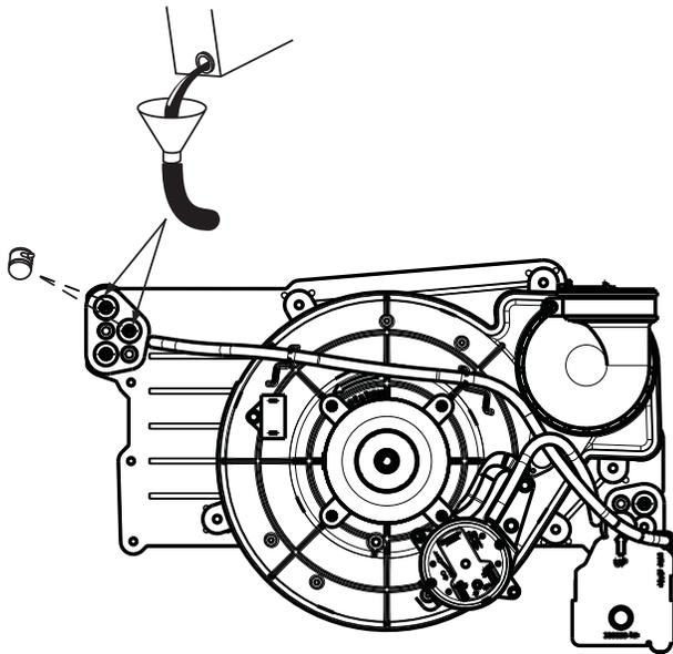
**Fig. 61 – Priming Condensate Trap**
