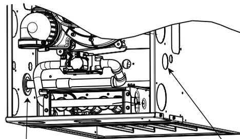
Gas Pipe Grommet Required For Direct Vent Applications
