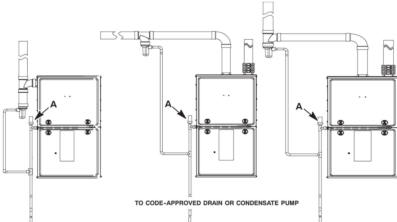
Recommend "T" fitting with 4-inch minimum height standpipe (A) of same diameter or larger extending upward.
