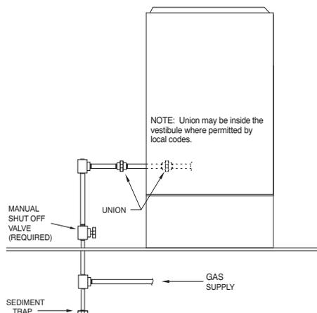
**Fig. 31 – Typical Gas Pipe Arrangement**
