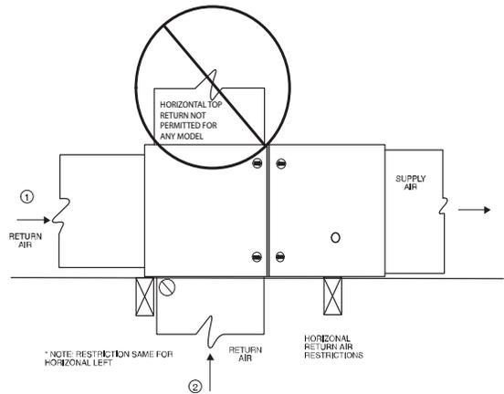
Fig. 22 – Horizontal Return Air Configurations and Restrictions
