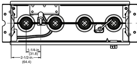
**Fig. 70 – Igniter Position - Top View**
