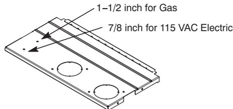
**Fig. 30 – Alternate Gas and Electric Entry**
