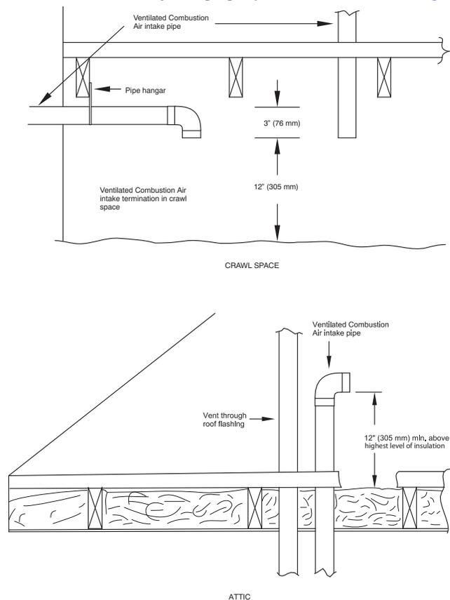
**Fig. 47 – Vent Terminations for Ventiladed Combustion Air**
