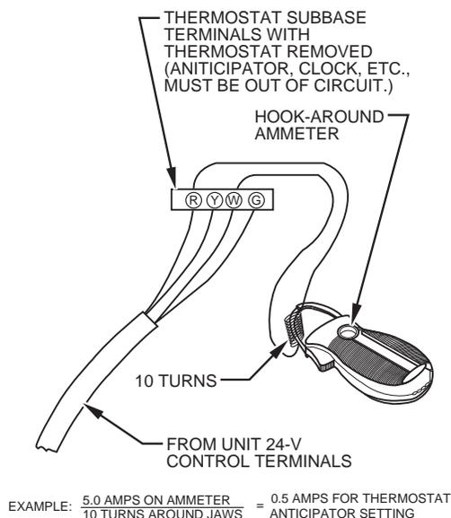
Fig. 66 – Amp. Draw Check with Ammeter
