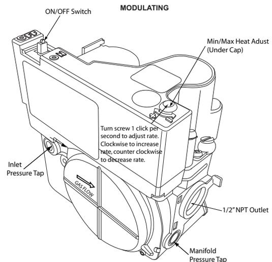
Fig. 64 – Gas Valve without Tower Pressure Ports
