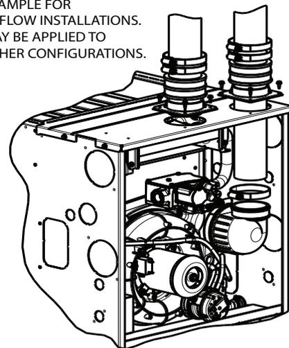
**Fig. 50 – Sample Inlet Air Pipe Connection for Polypropylene Venting Systems**
