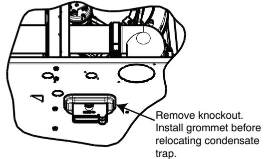
Fig. 17 – Horizontal Drain Trap Grommet
