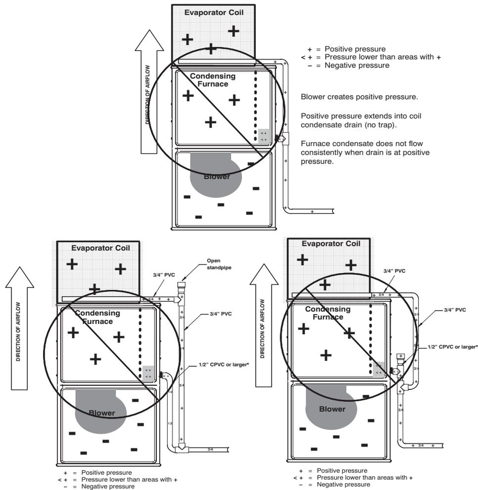
Fig. 12 – Example of Field Drain Attachment (Not Allowed)
